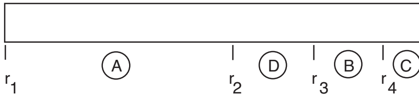
Figure 3-11 Spanwise specification of airfoil tables.
