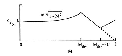
Figure 4-3. Airfoil characteristics -- moment coefficient and lift-curve slope.
