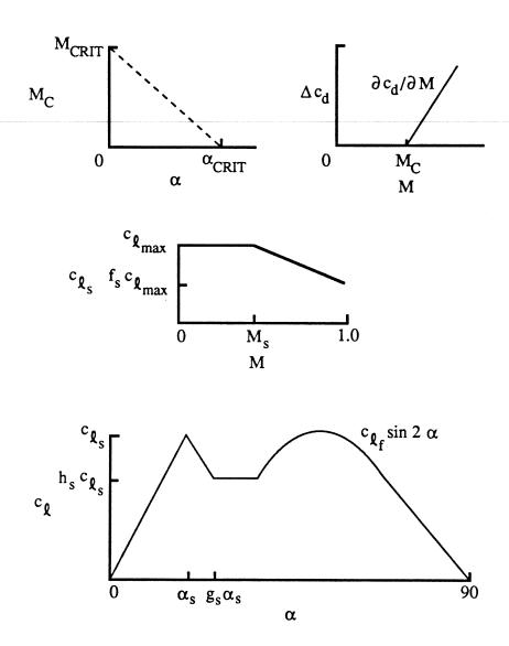
Figure 4-2. Airfoil characteristics -- lift and drag coefficients.
