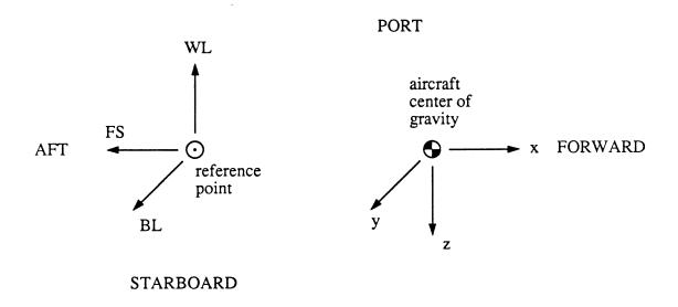
Figure 6-4. Definition of aircraft geometry.
