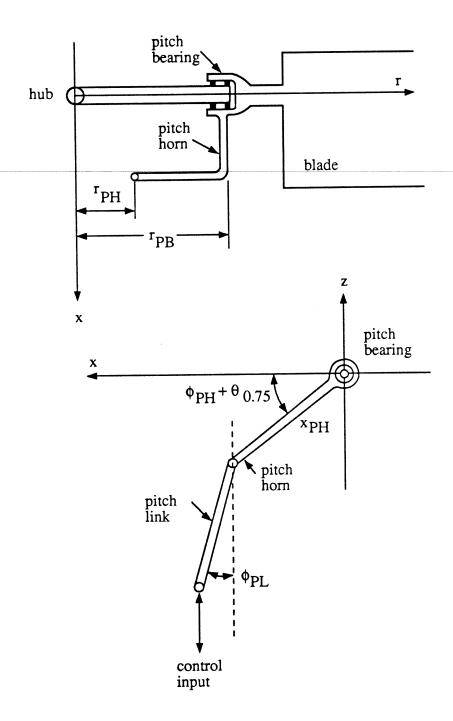
Figure 6-3. Schematic of blade root and control system geometry for calculation the kinematic pitch-bending coupling.
