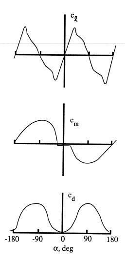
Figure 4-1. Sketch of section aerodynamic characteristics.
