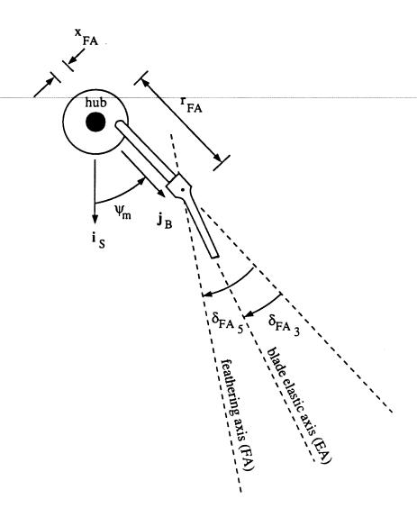
Figure 6-2. Schematic of the rotor hub and root geometry (top view).
