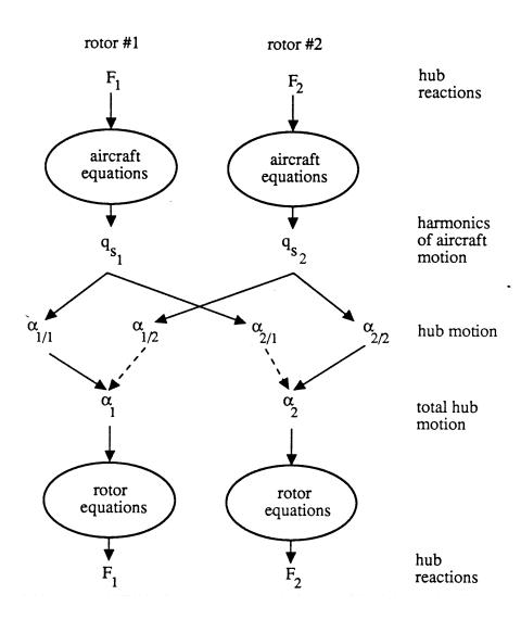
Figure 6-5. Outline of dynamic interaction of the two rotors.
