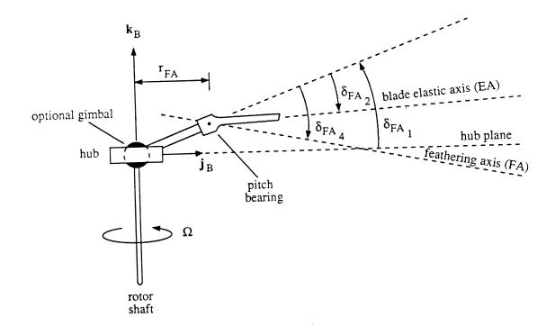
Figure 6-1. Schematic of the rotor hub and root geometry (side view).
