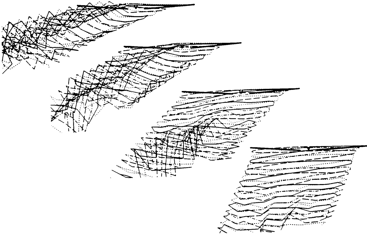
Figure 6. S-76 free wake geometry; C_T/\sigma = .08 , \alpha_s = -2 deg, \mu = .025 to .100 .
